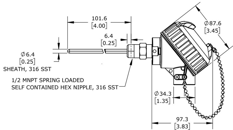
PROSENSE TEMPERATURE SENSOR, 10K-3 THERMISTOR, CONNECTION HEAD SPRING-LOADED PROBE, 4IN INSERTION LENGTH, 1/4IN PROBE DIAMETER, STAINLESS STEEL SHEATH, 1/2IN MALE NPT PROCESS CONNECTION, ALUMINUM SCREW COVER HEAD WITH 24IN, 24 AWG PVC WIRE LEADS
