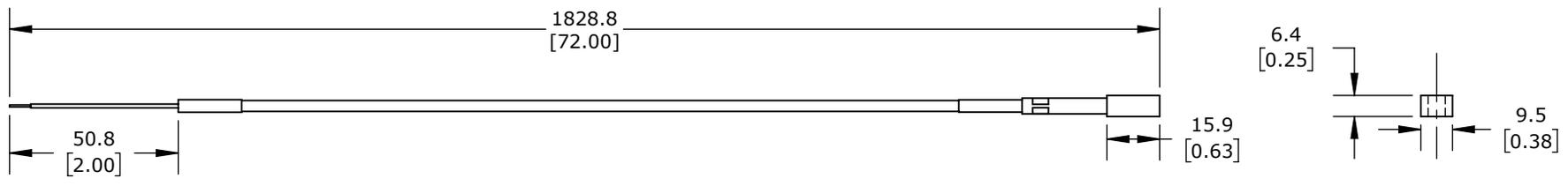
PROSENSE TEMPERATURE SENSOR, 10K-3 THERMISTOR, BOLT-ON RING, BRASS SHEATH, #6 TO #10 (4mm TO 5mm) SCREW OR BOLT SIZE PROCESS CONNECTION, 72IN, 24 AWG PVC WIRE LEADS
