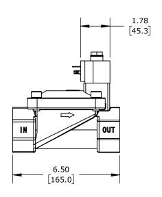
2-PORT (2-WAY), 2-POSITION, N.O., LEAD-FREE BRASS BODY, EPDM RUBBER SEAL(s), 2IN FEMALE NPT INLET(s), 2IN FEMALE NPT OUTLET(s), CV=48, 24 VDC OPERATING VOLTAGE, 9W, NSF/ANSI 61.
