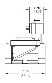
2-PORT (2-WAY), 2-POSITION, N.O., LEAD-FREE BRASS BODY, EPDM RUBBER SEAL(s), 1-1/2IN FEMALE NPT INLET(s), 1-1/2IN FEMALE NPT OUTLET(s), CV=30, 24 VDC OPERATING VOLTAGE, 9W, NSF/ANSI 61.
