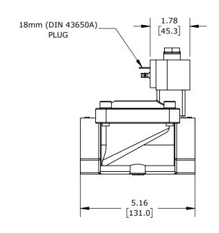
2-PORT (2-WAY), 2-POSITION, N.O., LEAD-FREE BRASS BODY, EPDM RUBBER SEAL(s), 1-1/4IN FEMALE NPT INLET(s), 1-1/4IN FEMALE NPT OUTLET(s), CV=22, 24 VDC OPERATING VOLTAGE, 9W, NSF/ANSI 61.
