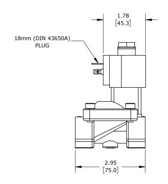
2-PORT (2-WAY), 2-POSITION, N.O., LEAD-FREE BRASS BODY, EPDM RUBBER SEAL(s), 3/4IN FEMALE NPT INLET(s), 3/4IN FEMALE NPT OUTLET(s), CV=6.7, 24 VDC OPERATING VOLTAGE, 9W, NSF/ANSI 61.
