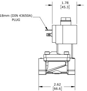
2-PORT (2-WAY), 2-POSITION, N.O., LEAD-FREE BRASS BODY, EPDM RUBBER SEAL(s), 1/2IN FEMALE NPT INLET(s), 1/2IN FEMALE NPT OUTLET(s), CV=4.3, 24 VDC OPERATING VOLTAGE, 9W, NSF/ANSI 61.
