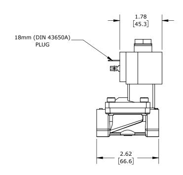
2-PORT (2-WAY), 2-POSITION, N.O., LEAD-FREE BRASS BODY, EPDM RUBBER SEAL(s), 3/8IN FEMALE NPT INLET(s), 3/8IN FEMALE NPT OUTLET(s), CV=4.3, 24 VDC OPERATING VOLTAGE, 9W, NSF/ANSI 61.
