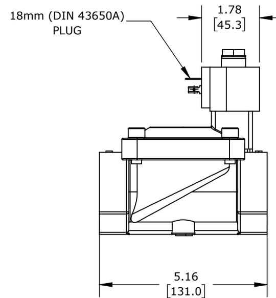
2-PORT (2-WAY), 2-POSITION, N.O., LEAD-FREE BRASS BODY, EPDM RUBBER SEAL(S), 1-1/4IN FEMALE NPT INLET(S), 1-1/4IN FEMALE NPT OUTLET(S), CV=22, 120 VAC OPERATING VOLTAGE, 8W, NSF/ANSI 61.
