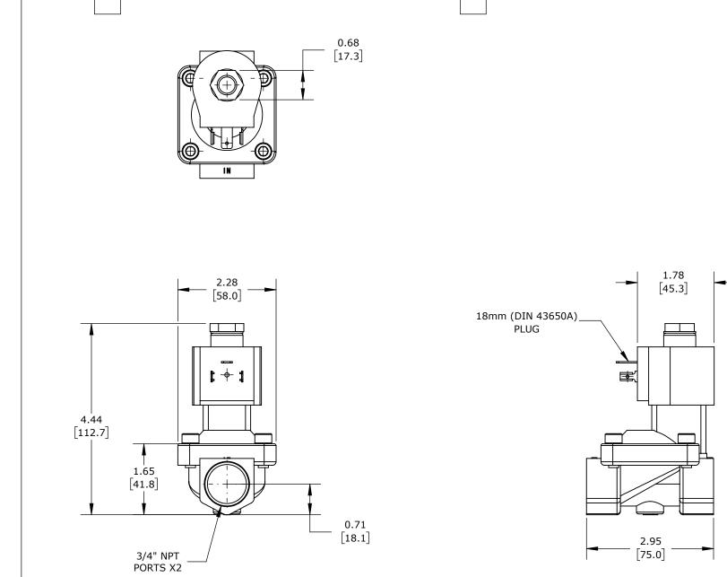
2-PORT (2-WAY), 2-POSITION, N.O., LEAD-FREE BRASS BODY, EPDM RUBBER SEAL(s), 3/4IN FEMALE NPT INLET(s), 3/4IN FEMALE NPT OUTLET(s), CV=6.7, 120 VAC OPERATING VOLTAGE, 8W, NSF/ANSI 61.
