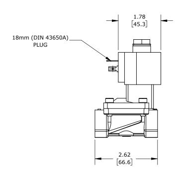
2-PORT (2-WAY), 2-POSITION, N.O., LEAD-FREE BRASS BODY, EPDM RUBBER SEAL(s), 3/8IN FEMALE NPT INLET(s), 3/8IN FEMALE NPT OUTLET(s), CV=4.3, 120 VAC OPERATING VOLTAGE, 8W, NSF/ANSI 61.
