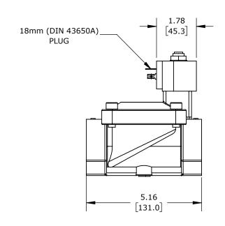
2-PORT (2-WAY), 2-POSITION, N.C., LEAD-FREE BRASS BODY, EPDM RUBBER SEAL(s), 1-1/2IN FEMALE NPT INLET(s), 1-1/2IN FEMALE NPT OUTLET(s), CV=30, 24 VDC OPERATING VOLTAGE, 9W, NSF/ANSI 61.
