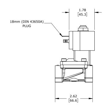
2-PORT (2-WAY), 2-POSITION, N.C., LEAD-FREE BRASS BODY, EPDM RUBBER SEAL(s), 1/2IN FEMALE NPT INLET(s), 1/2IN FEMALE NPT OUTLET(s), CV=4.3, 24 VDC OPERATING VOLTAGE, 9W, NSF/ANSI 61.
