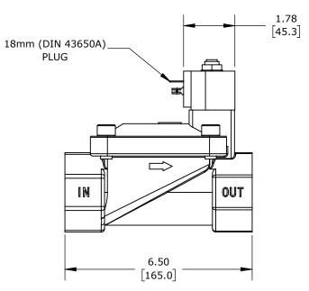
2-PORT (2-WAY), 2-POSITION, N.C., LEAD-FREE BRASS BODY, EPDM RUBBER SEAL(s), 2IN FEMALE NPT INLET(s), 2IN FEMALE NPT OUTLET(s), CV=48, 120 VAC OPERATING VOLTAGE, 8W, NSF/ANSI 61.
