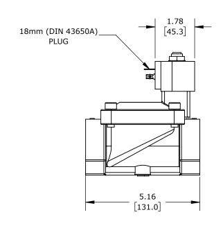
2-PORT (2-WAY), 2-POSITION, N.C., LEAD-FREE BRASS BODY, EPDM RUBBER SEAL(s), 1-1/4IN FEMALE NPT INLET(s), 1-1/4IN FEMALE NPT OUTLET(s), CV=22, 120 VAC OPERATING VOLTAGE, 8W, NSF/ANSI 61.
