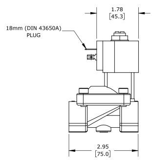
2-PORT (2-WAY), 2-POSITION, N.C., LEAD-FREE BRASS BODY, EPDM RUBBER SEAL(s), 3/4IN FEMALE NPT INLET(s), 3/4IN FEMALE NPT OUTLET(s), CV=6.7, 120 VAC OPERATING VOLTAGE, 8W, NSF/ANSI 61.
