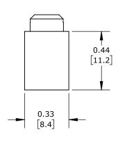
ALUMINUM-TIN PLATED, 5 OPENINGS, 4 CIRCUITS, MOUNTING HOLE POSITION 3, COPPER OR ALUMINUM, AL9CU.
