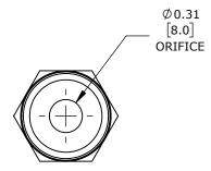
MALE, STRAIGHT, NICKEL PLATED BRASS BODY, NICKEL-PLATED BRASS THREADS, THREAD SEALANT, 3/8IN PUSH-TO-CONNECT TO 1/2IN NPT. PACKAGE OF 5.
