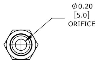
MALE, STRAIGHT, NICKEL PLATED BRASS BODY, NICKEL-PLATED BRASS THREADS, THREAD SEALANT, 1/4IN PUSH-TO-CONNECT TO R1/8 BSPT. PACKAGE OF 5.
