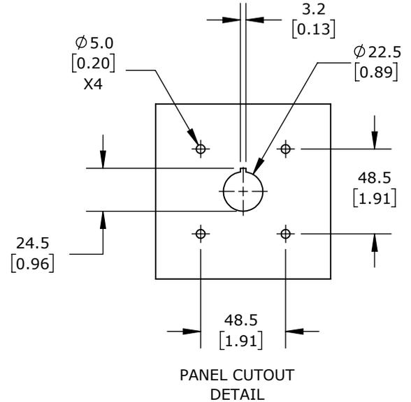
SELECTOR, BLACK/GRAY, EXTERNAL FRONT MOUNT, 2-POSITION, LOCKABLE IN OFF ONLY, DEFEATABLE, NEMA 4/4X, IP65. FOR USE WITH MPW80 SERIES MANUAL MOTOR PROTECTORS. 330mm SHAFT INCLUDED.
