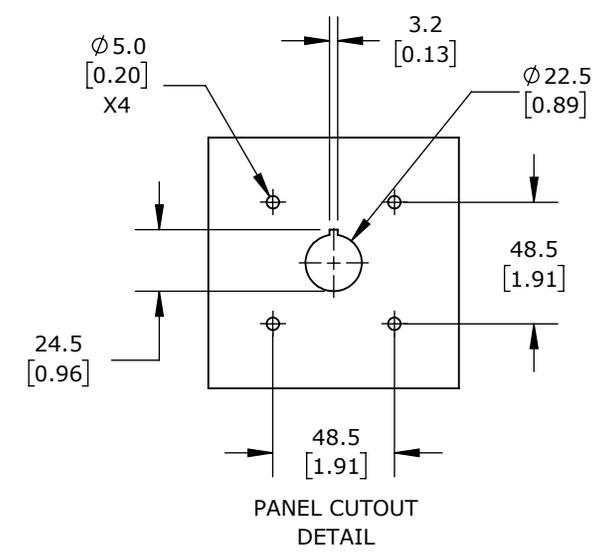
SELECTOR, RED/YELLOW, EXTERNAL FRONT MOUNT, 2-POSITION, LOCKABLE IN OFF ONLY, DEFEATABLE, NEMA 4/4X, IP65. FOR USE WITH MPW80 SERIES MANUAL MOTOR PROTECTORS. 130mm SHAFT INCLUDED.
