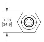
0.1-7 GPM, 3/8IN NPT THREAD, ANODIZED ALUMINUM.
