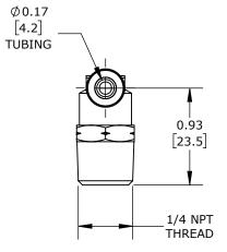
MALE, ELBOW, ROTATING, NICKEL PLATED BRASS BODY, NICKEL-PLATED BRASS THREADS, THREAD SEALANT, 5/32IN (4MM) PUSH-TO-CONNECT TO 1/4IN NPT. PACKAGE OF 5.
