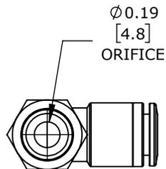
MALE, ELBOW, ROTATING, NICKEL PLATED BRASS BODY, NICKEL-PLATED BRASS THREADS, THREAD SEALANT, 1/4IN PUSH-TO-CONNECT TO R1/8 BSPT. PACKAGE OF 5.
