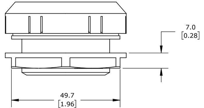
M40 X 1.5MM THREAD TYPE, POLYAMIDE, LIGHT GRAY, 6250 ML/MIN @ 70 mbar (1 PSI), IP66 IP68, UL TYPE 4X. PACKAGE OF 2.
