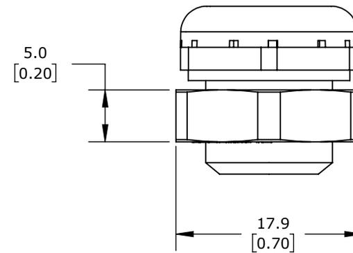
M12 X 1.5MM THREAD TYPE, POLYAMIDE, BLACK, 417 ML/MIN @ 70 mbar (1 PSI). PACKAGE OF 2.
