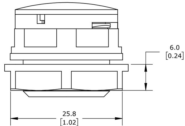
M20 X 1.5MM THREAD TYPE, POLYAMIDE, BLACK, 2000 ML/MIN @ 70 mbar (1 PSI), IP66 IP68. PACKAGE OF 2.
