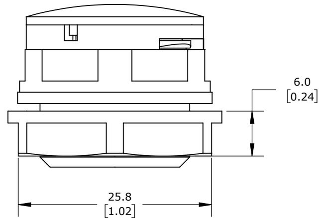
M20 X 1.5MM THREAD TYPE, POLYAMIDE, LIGHT GRAY, 2000 ML/MIN @ 70 mbar (1 PSI), IP66 IP68. PACKAGE OF 2.
