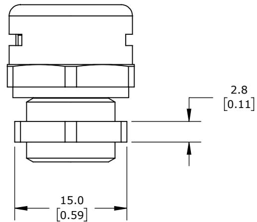
M12 X 1.5MM THREAD TYPE, STAINLESS STEEL, 417 ML/MIN @ 70 mbar (1 PSI), IP66 IP68, UL TYPE 4X. PACKAGE OF 1.
