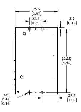
EVER MOTION SOLUTIONS DC OPEN/CLOSED LOOP MICROSTEPPING STEPPER DRIVE, 10A PER PHASE, 2-PHASE OUTPUT, 24-75 VDC, BIPOLAR, POSITION MODE, 200 TO 65536 STEPS PER REVOLUTION, (1) 4-PIN TERMINAL PORT(s). REQUIRES LW4D3KIT-CO CONNECTOR KIT OR LW4D3KIT-050 CABLE KIT
