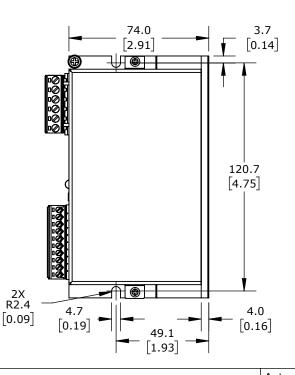
EVER MOTION SOLUTIONS DC OPEN LOOP MICROSTEPPING STEPPER DRIVE, 10A PER PHASE, 2-PHASE OUTPUT, 24-80 VDC, BIPOLAR, POSITION MODE, 200 TO 51200 STEPS PER REVOLUTION
