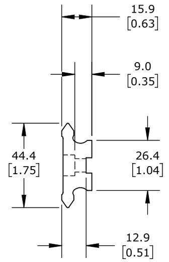
HIGH CARBON STEEL (HCS), 16 X 44 X 716mm.
