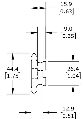
HIGH CARBON STEEL (HCS), 16 X 44 X 536mm.
