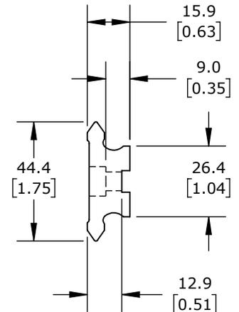
HIGH CARBON STEEL (HCS), 16 X 44 X 1256mm.
