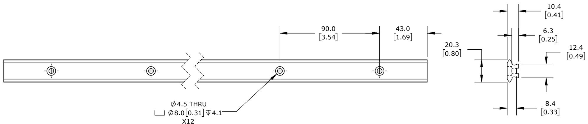
HIGH CARBON STEEL (HCS), 10 X 20 X 1076mm.
