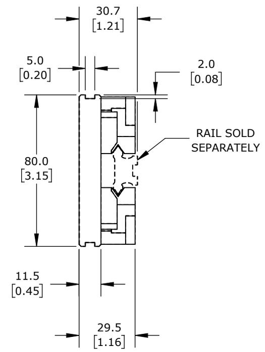
DOUBLE ROW BALL BEARING, END SEAL, ANODIZED ALUMINUM/STEEL.
