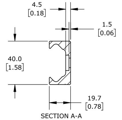
ANODIZED ALUMINUM, 19.74 X 40 X 1520mm. FOR USE WITH SUREMOTION LUV-2 SERIES V-CARRIAGES.
