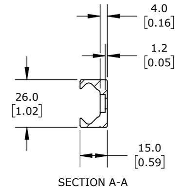
ANODIZED ALUMINUM, 15 X 26 X 800mm. FOR USE WITH SUREMOTION LUV-1 SERIES V-CARRIAGES.
