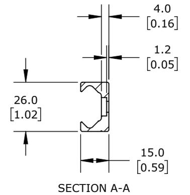
ANODIZED ALUMINUM, 15 X 26 X 640mm. FOR USE WITH SUREMOTION LUV-1 SERIES V-CARRIAGES.
