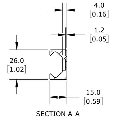
ANODIZED ALUMINUM, 15 X 26 X 480mm. FOR USE WITH SUREMOTION LUV-1 SERIES V-CARRIAGES.
