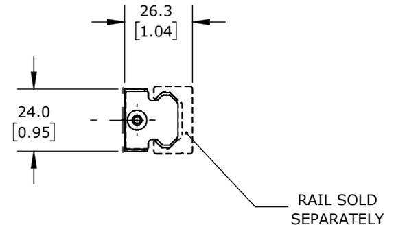
SINGLE ROW BALL BEARING, END SEAL, POLYACETAL/440C STAINLESS STEEL.
