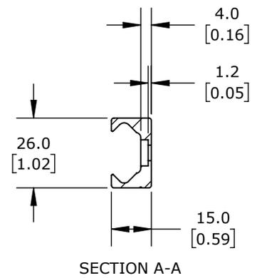
ANODIZED ALUMINUM, 15 X 26 X 1520mm. FOR USE WITH SUREMOTION LUV-1 SERIES V-CARRIAGES.
