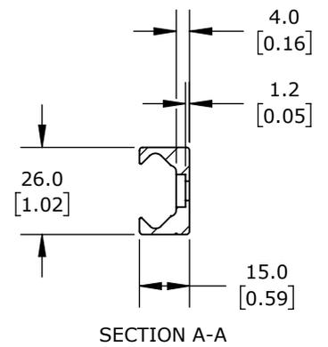
ANODIZED ALUMINUM, 15 X 26 X 1280mm. FOR USE WITH SUREMOTION LUV-1 SERIES V-CARRIAGES.
