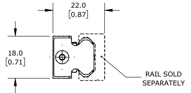
SINGLE ROW BALL BEARING, END SEAL, POLYACETAL/440C STAINLESS STEEL.
