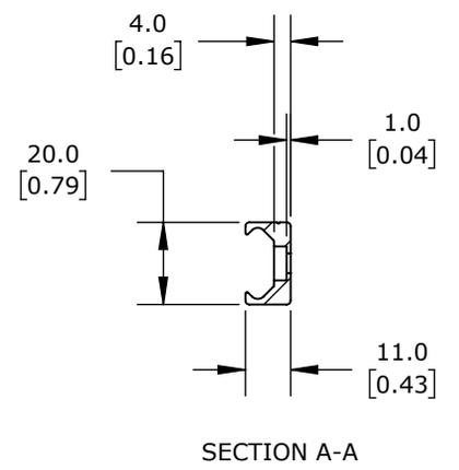
ANODIZED ALUMINUM, 11 X 20 X 1120mm. FOR USE WITH SUREMOTION LUV-0 SERIES V-CARRIAGES.
