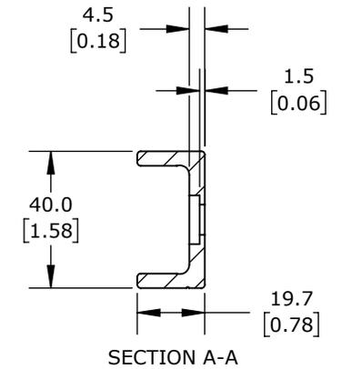
ANODIZED ALUMINUM, 19.74 X 40 X 640mm. FOR USE WITH SUREMOTION LUC-2 SERIES CROWN CARRIAGES.
