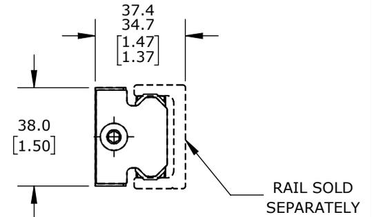
SINGLE ROW BALL BEARING, END SEAL, POLYACETAL/440C STAINLESS STEEL. FOR USE WITH SUREMOTION LUC-2 SERIES GUIDE TRACKS.
