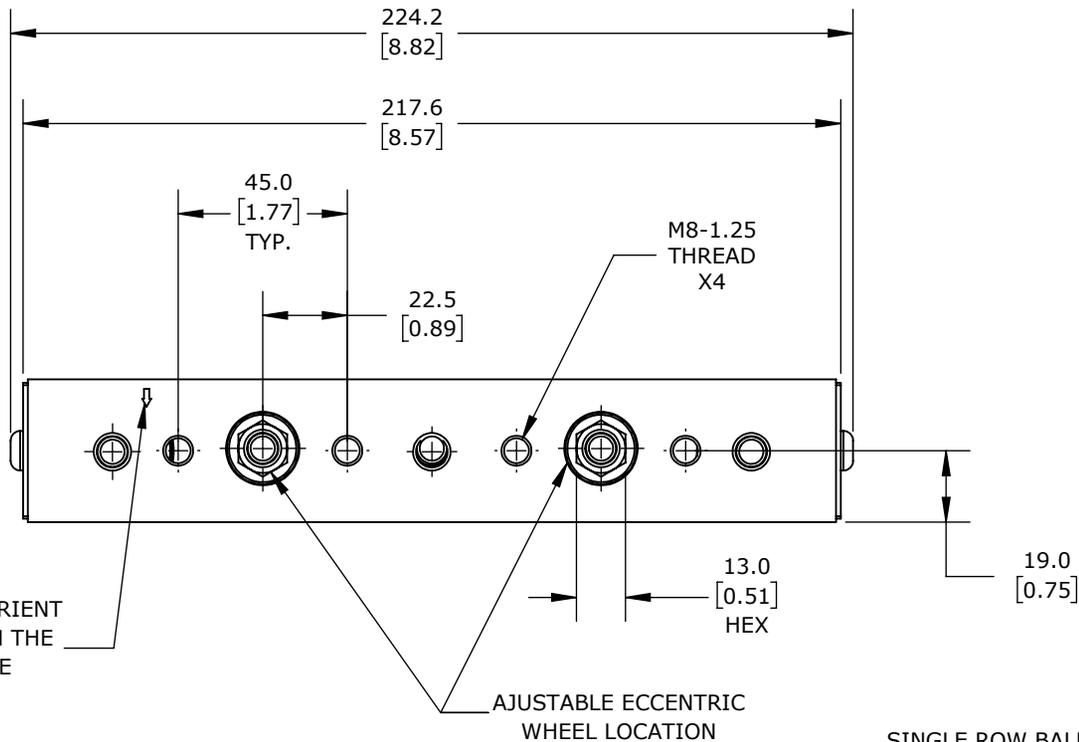
WHEN INSTALLING, ORIENT EMBOSSED ARROW IN THE DIRECTION OF THE APPLIED LOAD
