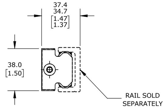
SINGLE ROW BALL BEARING, END SEAL, POLYACETAL/440C STAINLESS STEEL.
