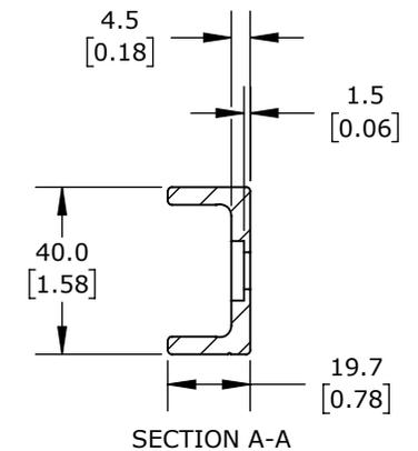
ANODIZED ALUMINUM, 19.74 X 40 X 1280mm. FOR USE WITH SUREMOTION LUC-2 SERIES CROWN CARRIAGES.
