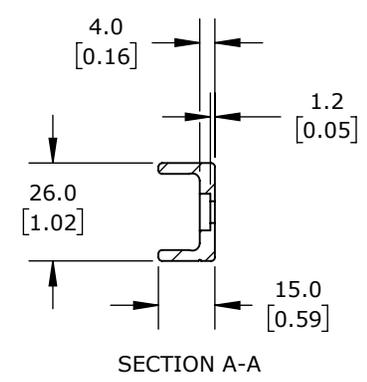
ANODIZED ALUMINUM, 15 X 26 X 960mm. FOR USE WITH SUREMOTION LUC-1 SERIES CROWN CARRIAGES.
